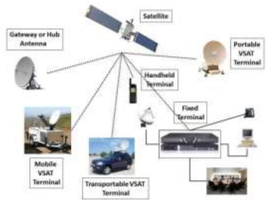
Figure 3. Satellite Communication Architecture for Disaster Management
